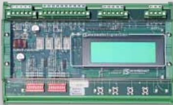
sm electrics' A067 *mtBUS* controller is designed to manage and monitor permanently all connected network units. Simply to be mounted on a terminal rail (TS35) the controller provides useful system information to the commissioning, service and maintenance staff indicated clearly on a 4 lines 20 characters LC display.
